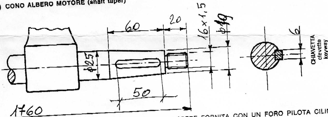
SE LE MISURE NON SONO NOTE, L'ELICA PUO' ESSERE FORNITA CON UN FORO PILOTA CILINDRICO (If the measures are not known, the propeller can be supplied with a cylindrical pilot bore).
